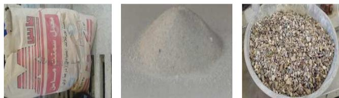
Fig. 1 Cement, fine aggregate and coarse aggregate.
