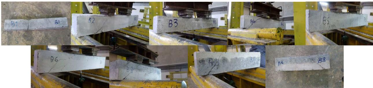
Fig. 10 Shear failure and crack propagations of the tested beams
