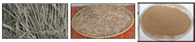
Fig. 1. Rice straw physical pretreatment (a). Rice straw (b). Drying process (Sun-dry) (c) rice straw powder 200 mesh.
