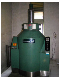
Fig. 1. Irradiator ^{60}\text{Co} Gammacell 220 at PATIR BATAN
