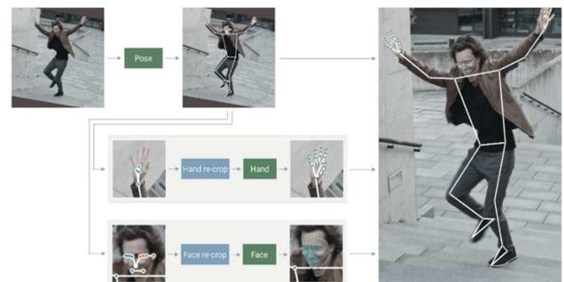
Fig. 2 Position hands, Pose, and face detection display.
