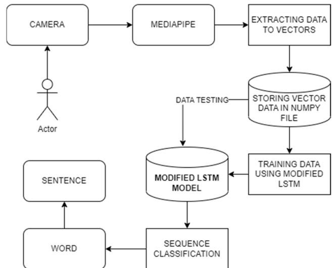
Fig. 1 Proposed diagram system for continuous SLR using Mediapipe and Modified LSTM
