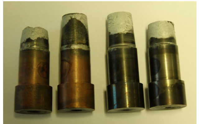
Fig. 2: Optical photograph of core pins after HPDC trials from left to right: bi-metallic short, bi-metallic long, tool steel long and tool steel short
