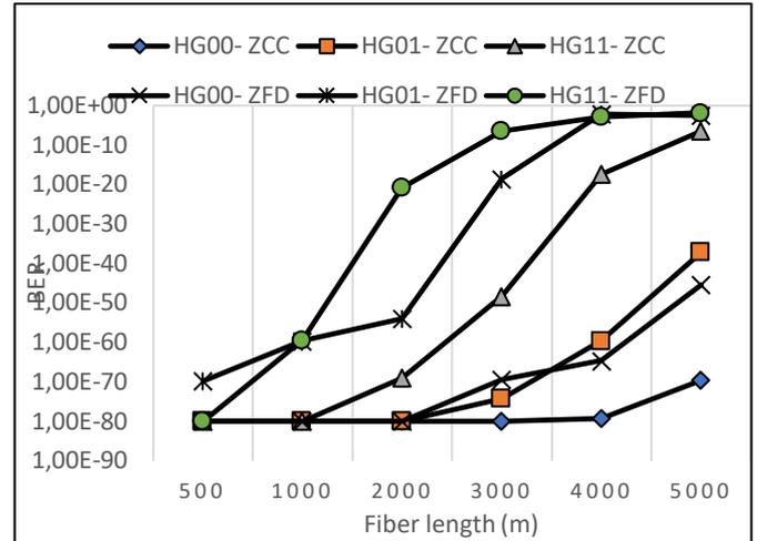
Fig. 5 BER versus fibre length
