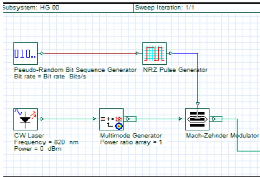
Fig. 4 Data generation of HG00 mode
