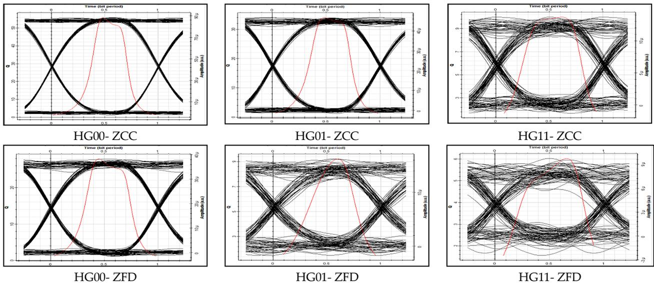
Fig. 8 Eye diagram at 4.5 km (5 Gbit/s)
