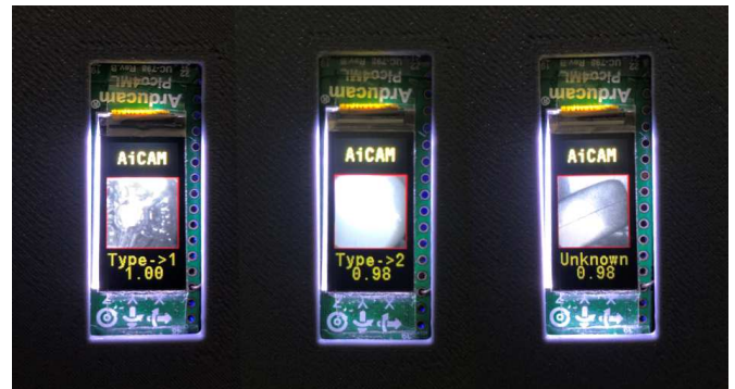
Fig. 15 The trained model's real-time performance on the Arduicam Pico 4ML embedded device
