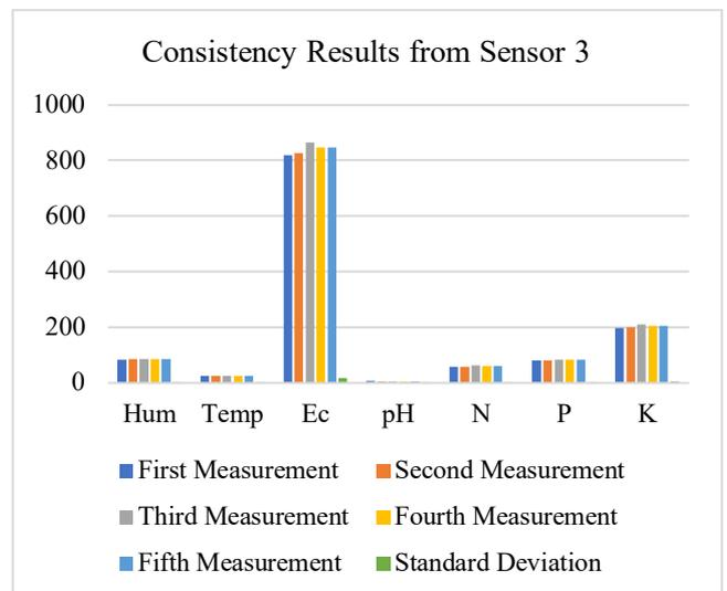
Fig. 14 Consistency measurement results from Sensor 3
