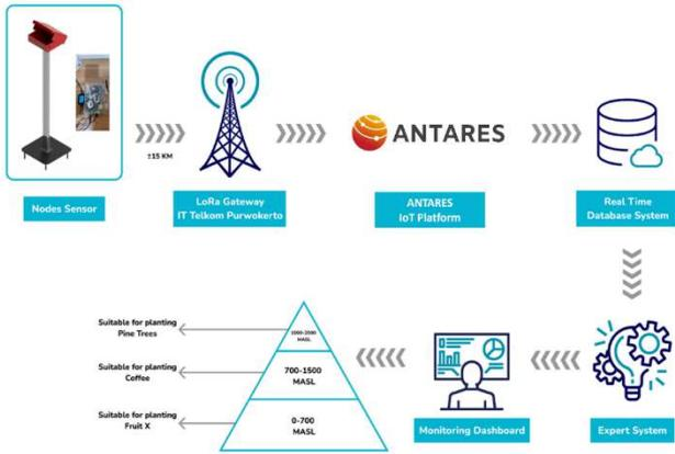
Fig. 2 Network configuration between the LoRa WAN and the Antares platform
