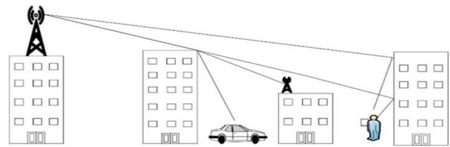
Fig. 1 Model propagation for LoRA communications with path loss, shadowing, and multipath [31]
