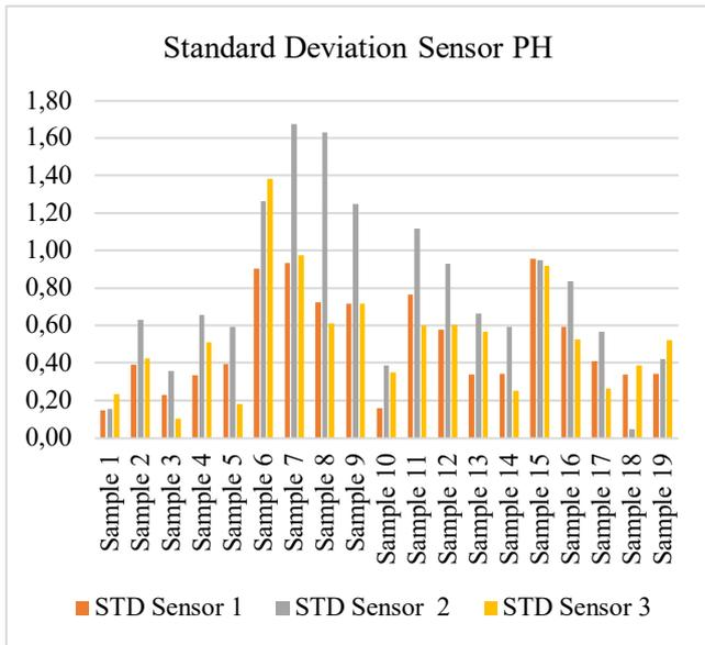
Fig. 11 Standard deviation values of pH from the three sensors
