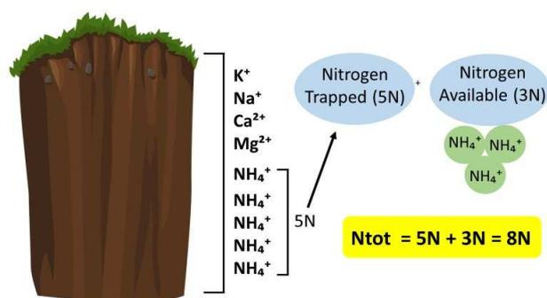
Fig. 15 Illustration of nitrogen trapped in the sensor test results and nitrogen available in the laboratory test results
