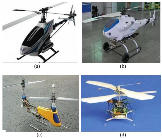
Fig. 1 Single-mode UAVs on the air operation. (a) Conventional main and tail rotor, (b) X - Copter1 by Skytech's, (c) Tandem and (d) \mu FR by Chiba University and Epson
