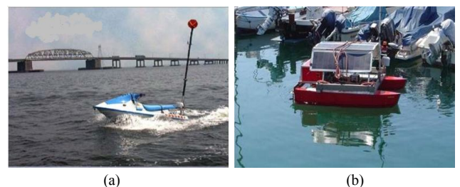
Fig. 3. Single-mode USVs on water surface operation, (a) X-Class USV and (b) Charlie USV
