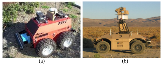
Fig. 2. Single-mode UGVs on the ground locomotion (a) ATRV, (b) MDARS
