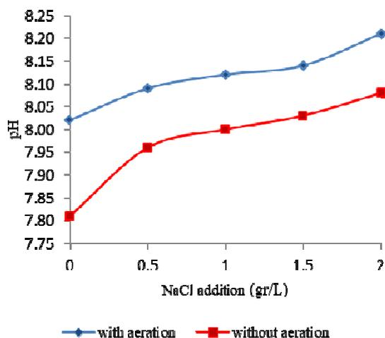
Fig. 2 Effect of aeration processes and NaCl concentration on pH
