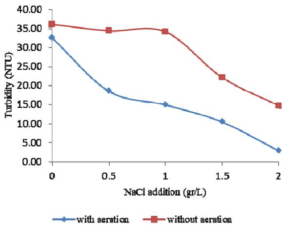
Fig. 7 Effect of aeration processes and NaCl addition to turbidity
