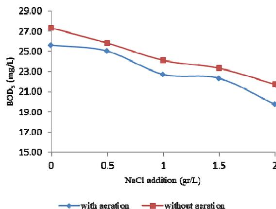
Fig. 6 Effect of aeration processes and NaCl concentration on BOD5
