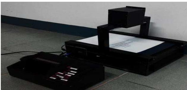
Fig. 2 The system set-up used in the study showing the braille platform and the image capturing device.
