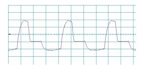
Fig. 10 main swith current (sampled with CT & oscilloscope)
