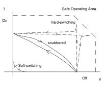
Fig. 1 Switching Diagram(hard switching and soft switching)
