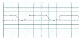
Fig. 11 main swith gate pulse (sampled with oscilloscope)
