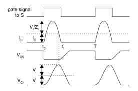
Fig. 3 Waveforms of resonant Dc to Dc step down converter(fig2)
