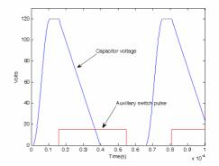
Fig. 7 simulation of resonant capacitor voltage
