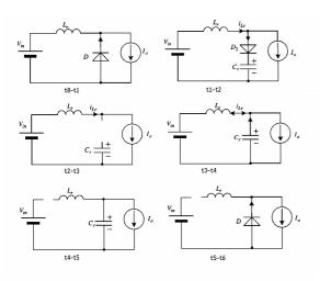
Fig. 5 six intervals of a cycle
