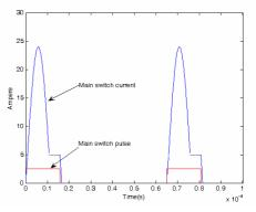
Fig. 8 simulation of main swith current
