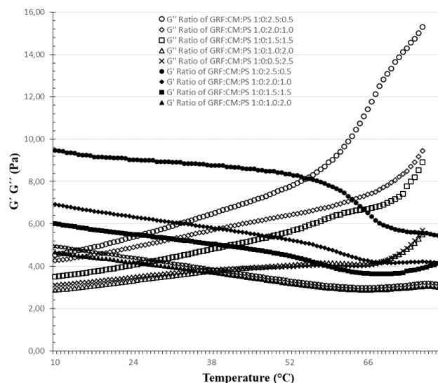
Fig 3. Storage modulus ( $G'$ ) and loss modulus ( $G''$ ) of ternary paste (GRF-CM-PS paste) as a function of temperature.  $G'$  filled symbols,  $G''$  empty symbols. The oscillatory rheometer was run at a cooling rate of 20°C/min; frequency of 0.4 Hz; strain amplitude of 0.2%.
