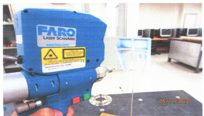
Fig. 1 Fish-head scanning using Faro Laser ScanArm
