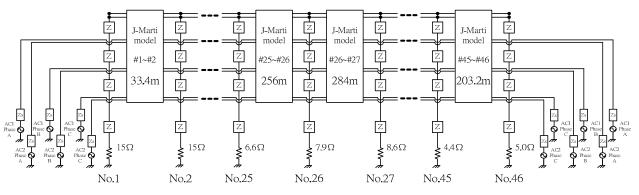
Fig. 5 Equivalent circuit for the selected transmission system
