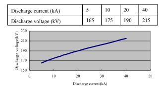
Fig. 4 V-I characteristic curve of line arrester
