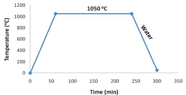
Fig 2. Normal of the heat treatment process
