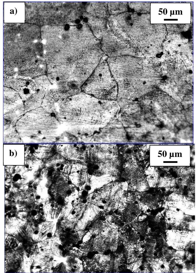
Fig 11. The microstructure of sample B-1. a) Before impact load b) After impact load
