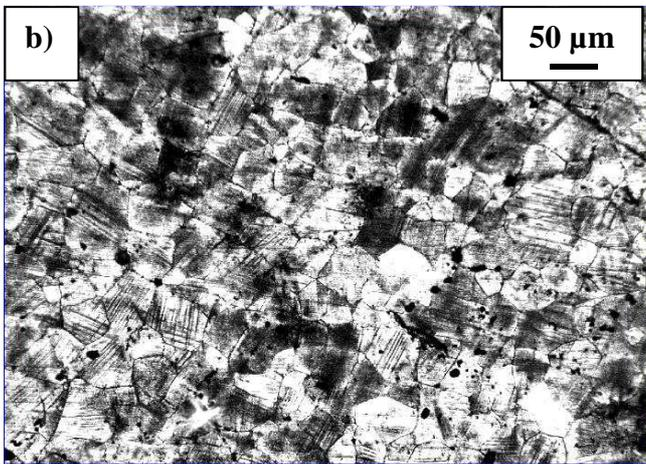
Fig 12. The microstructure of sample B-2. a) Before impact load b) After impact load
