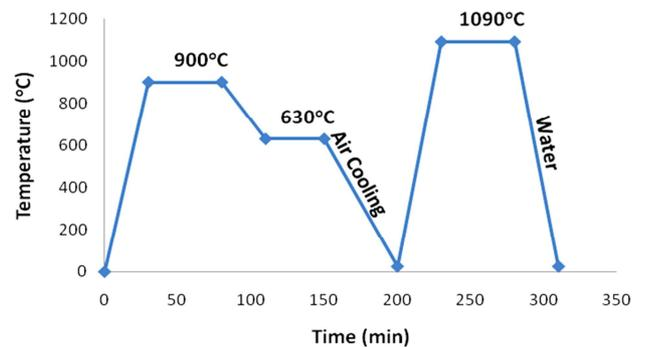
Fig 3. Model of the heat treatment process
