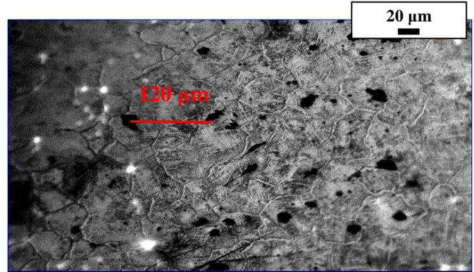
Fig 7. Microstructure of sample A-3 with Normal heat treatment process
