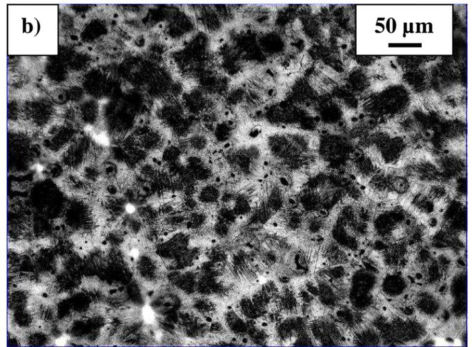
Fig 13. The microstructure of sample B-3. a) Before impact load b) After impact load
