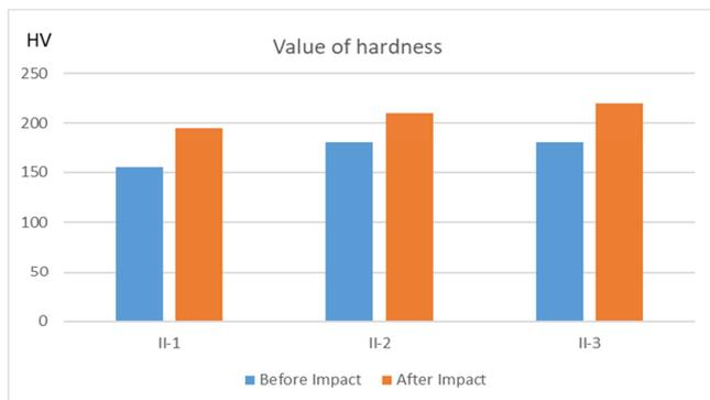
Fig 10. The hardness of samples type B with New heat treatment process
