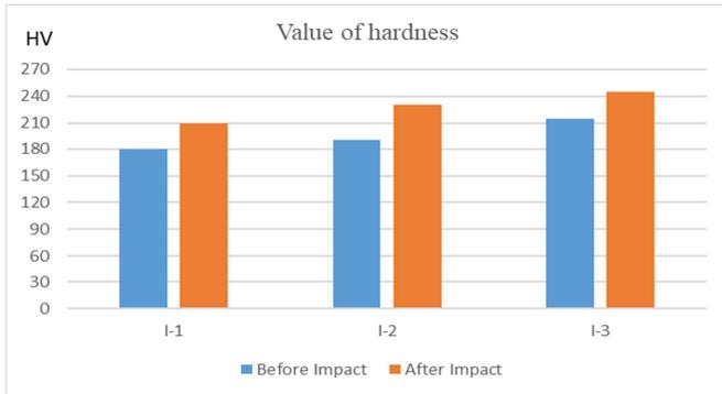
Fig. 4. The hardness of samples type A with Normal heat treatment process.
