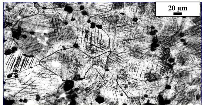
Fig 8. The microstructure of sample A-1 after impact load
