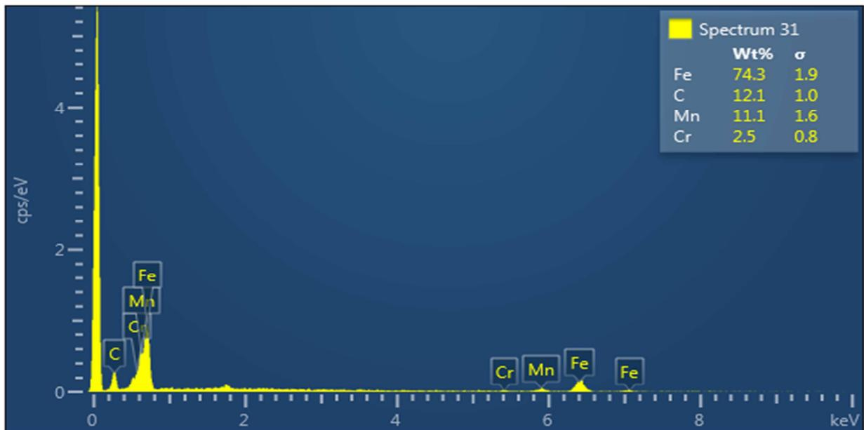
Fig 15. EDS of sample B-2 – after heat treatment
