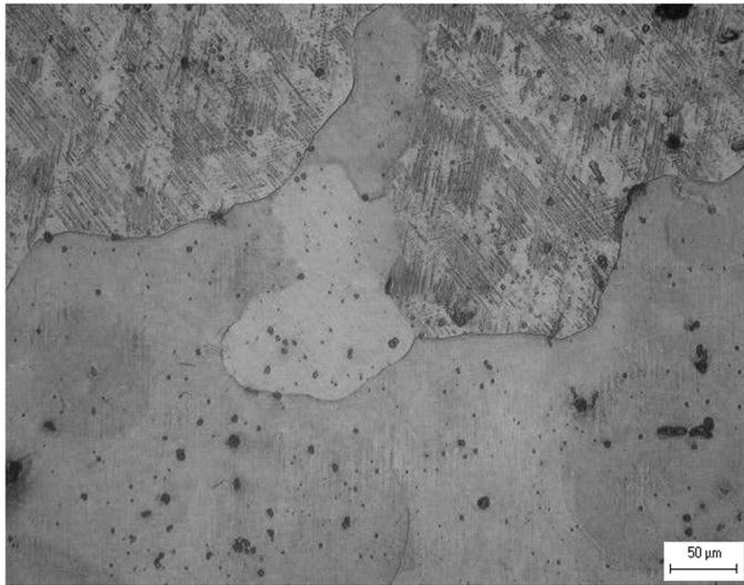
Fig 9. The microstructure of sample A-3 with new heat treatment process
