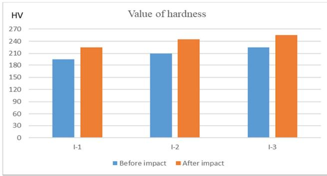
Fig 5. The hardness of samples type A with new heat treatment process
