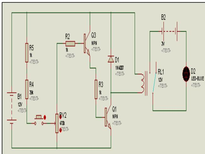
Fig. 10 Water sensor detector circuit
