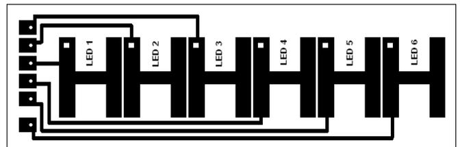
Fig. 4 Sensors for water level indicator unit
