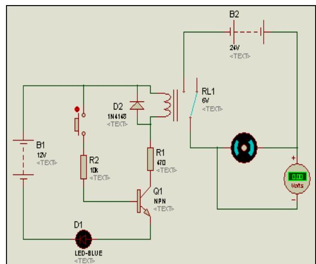
Fig.12 PLC interface schematic circuit
