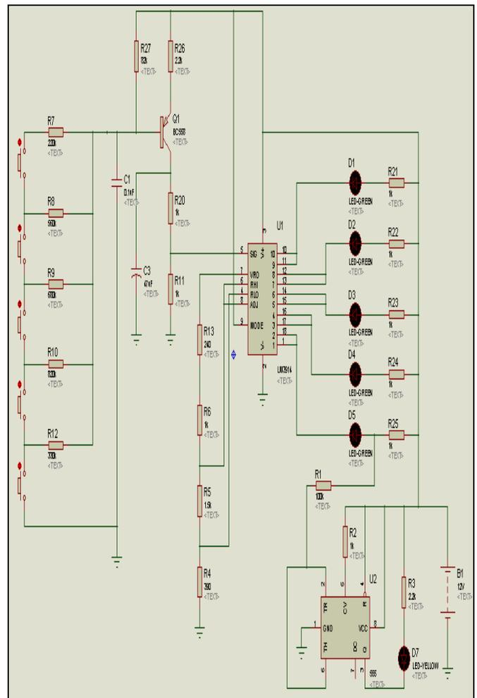
Fig. 8 Water level indicator schematic circuit
