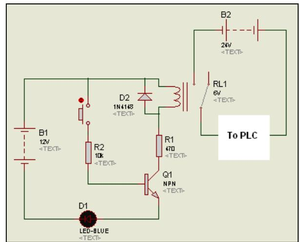
Fig. 5 Interface circuit for relay
