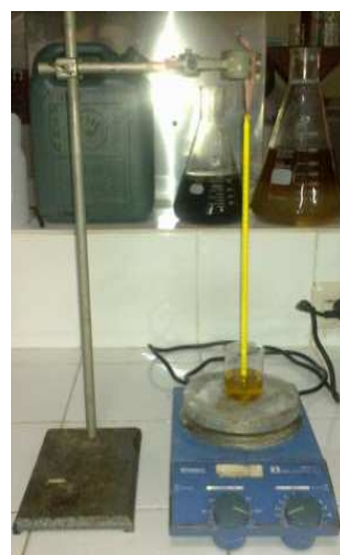
Fig. 4 Trophy glass for measure the smoke point
