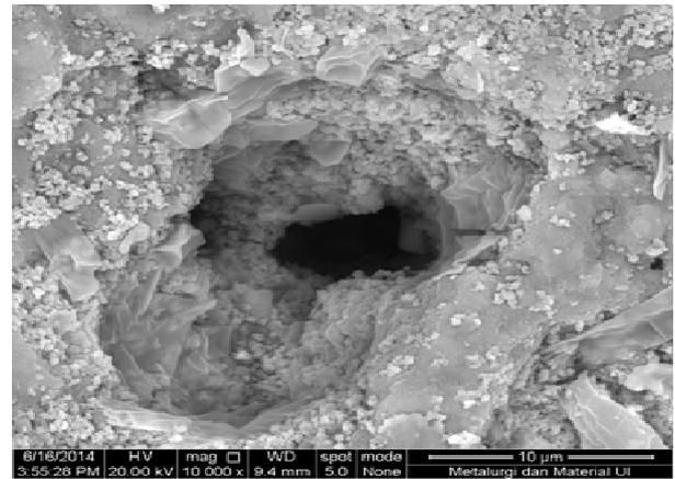
Fig.7 Fracture surface of Al/Al<sub>2</sub>O<sub>3</sub> composites taken from the tensile sample with 15wt-% Mg and 15 vf-% Al<sub>2</sub>O<sub>3</sub>.
