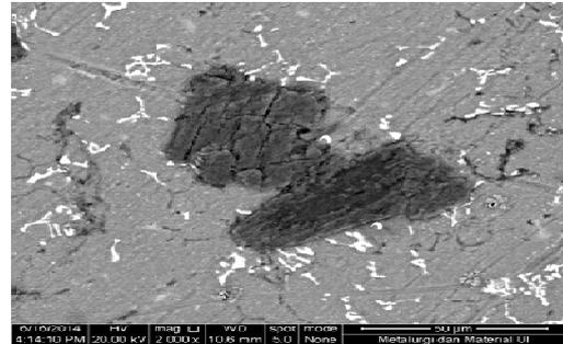
Fig. 6 SEM micrograph of Al/Al<sub>2</sub>O<sub>3</sub> composite with 10 vf-% Al<sub>2</sub>O<sub>3</sub>-10 wt-% Mg link to EDS to identify phase presence in composite
