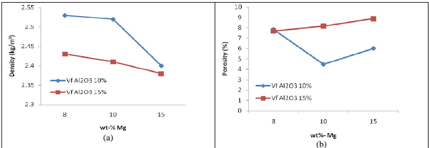
Fig. 2 Effect of Mg on density (a) and porosity (b) of Al6061/Al<sub>2</sub>O<sub>3</sub> metal matrix composites produced by double blade stir casting.
