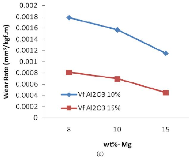
Fig.1 Effect of Mg on mechanical properties of Al6061/Al<sub>2</sub>O<sub>3</sub> metal matrix composites produced by double blade stir casting. a) Tensile strength, b) Hardness, c) Wear rate.
