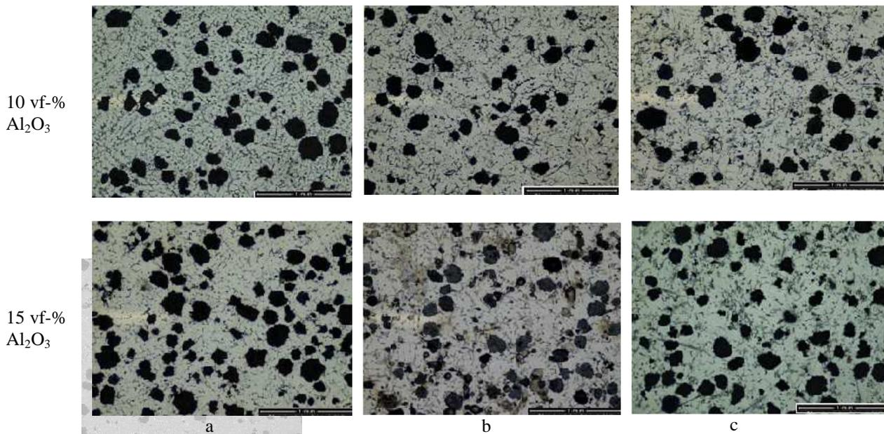
Fig. 3 Distribution of  $\text{Al}_2\text{O}_3$  particles with different Mg and  $\text{Al}_2\text{O}_3$  content in an Al 6061 matrix on metal matrix composites produced by double blade stir casting. a) 8wt-% Mg, b) 10 wt-% Mg and c) 15wt-% Mg
