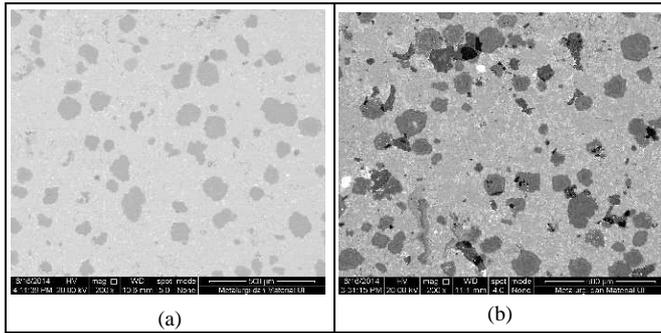
Fig.5 SEM micrograph of Al/Al<sub>2</sub>O<sub>3</sub> composite with 10 vf-% Al<sub>2</sub>O<sub>3</sub>-10 wt-% Mg (a) and (b) microstructure of Al/Al<sub>2</sub>O<sub>3</sub> composite with 15 vf-% Al<sub>2</sub>O<sub>3</sub>-15 wt% Mg
