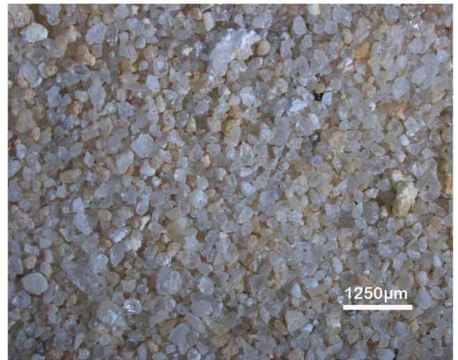
Fig. 2 Quartz grains overview under a microscope
