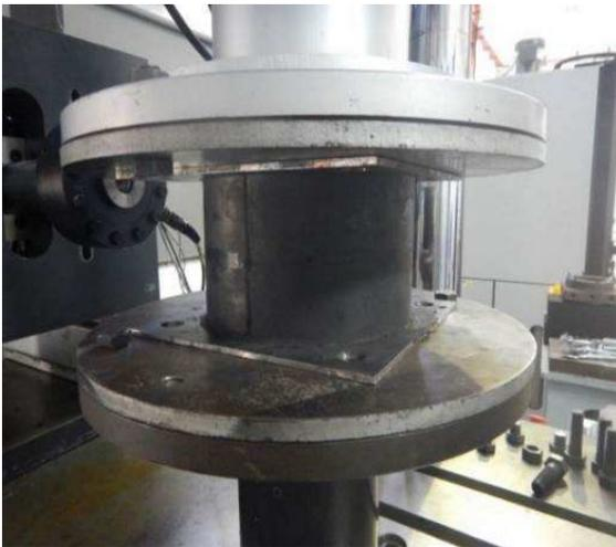
Fig. 7 Vertical test setup on MTS 322 servo-hydraulic machine
