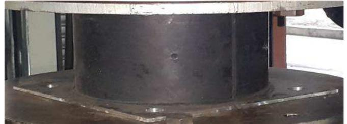
Fig. 16 Vertical-test sample A1 at the vertical displacement of 28 mm
