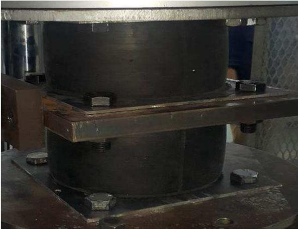
Fig. 13 Bulging effect of samples B1 and B2 in horizontal test
