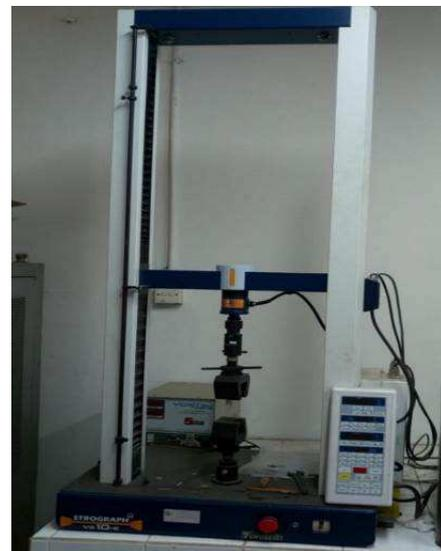
Fig. 5 Glass fiber tension test
