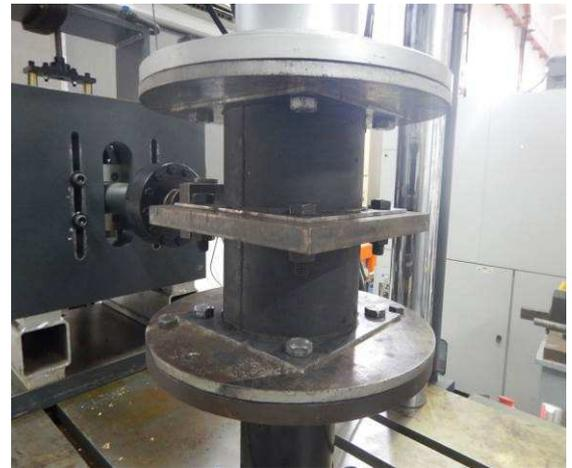
Fig. 9 Horizontal test setup on MTS 322 servo-hydraulic machine
