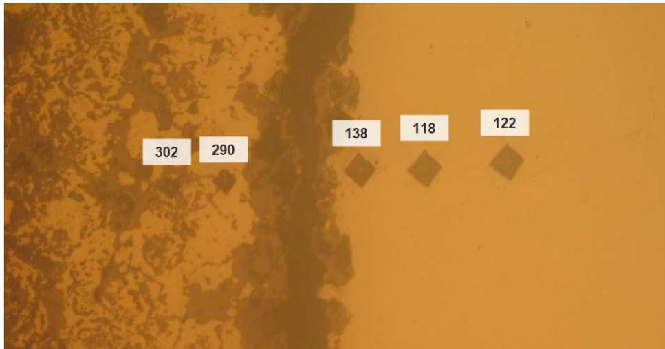
Fig. 11. The hardness value of the sample after heat treatment
