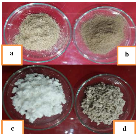
Fig. 3 Visual Appearances of Samples (a.) OPEFB Fibers, (b.) Mesocarp (c.) OPEFB \alpha -cellulose, (d.) Mesocarp \alpha -cellulose
