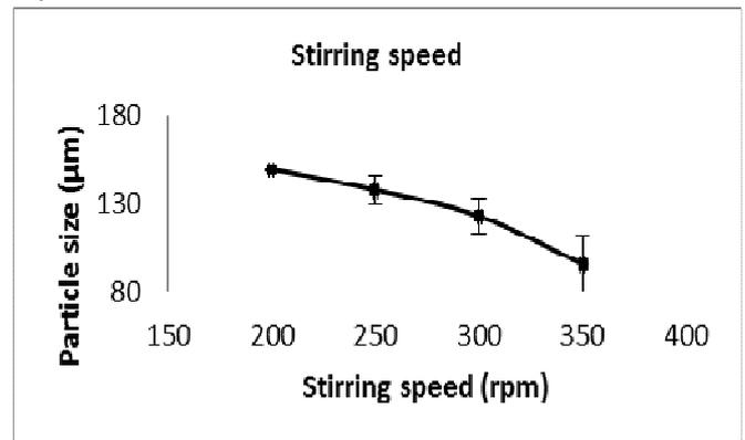
Fig. 6 Effect of stirring speed on microcarrier particle size
