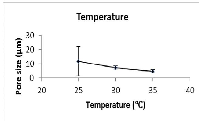
Fig. 8 Effect of temperature on microcarrier pore size
