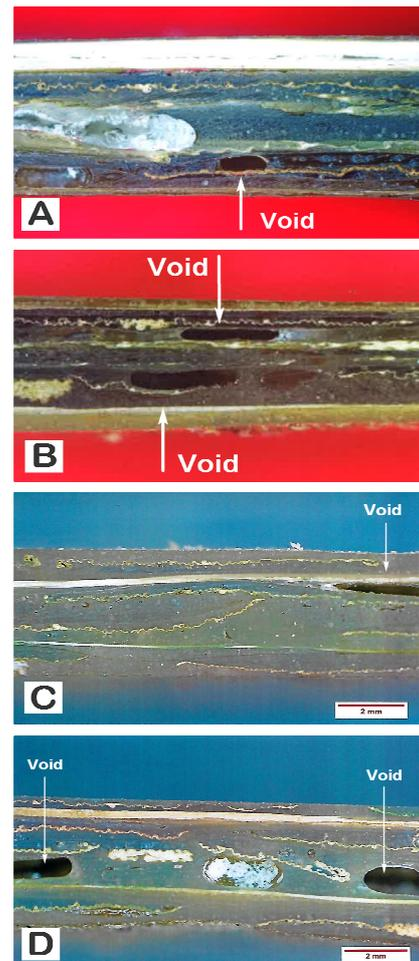
Fig. 3 Cross-sectioned microscopic structure of the RSF-reinforced polymer composite at 10% (A), 20% (B), 30% (C) and 40% (D) fibre loading (RSF<sub>NaOH</sub>).
