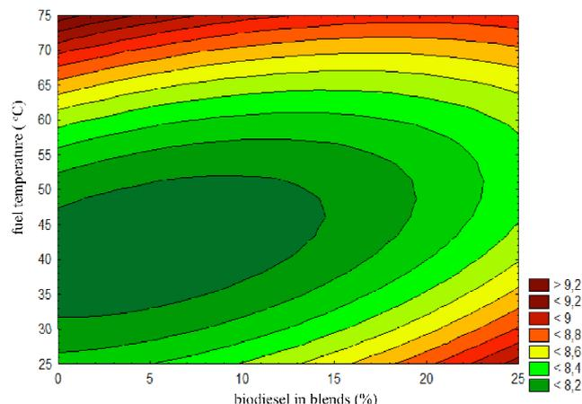
Fig. 3. Effects of Fuel Heating Temperature to Fuel Consumption
