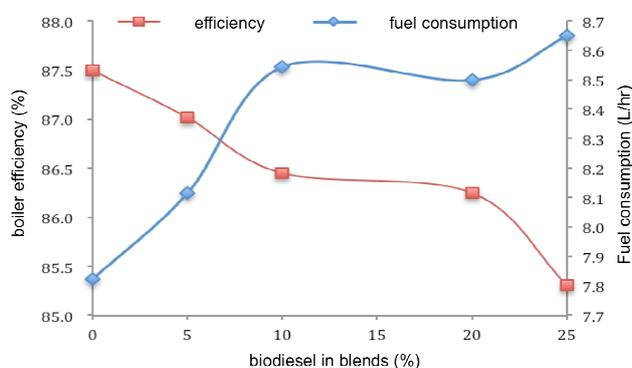
Fig. 2. Effects of BXX use on boiler performance at Business as Usual (BAU) condition
