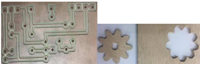
Fig. 5 PCB fabrication (left) and cut through plywood (right)
