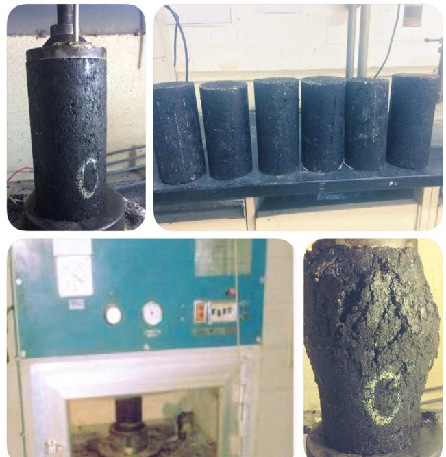
Fig. 8 Uniaxial repeated loading test
