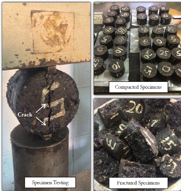
Fig. 5 Indirect tensile strength test
