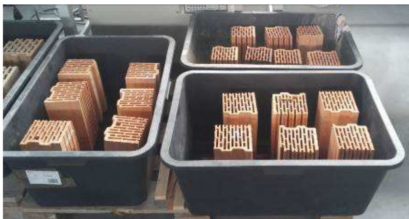
Fig. 2. Testing of hydrophobisation for ceramic masonry blocks.
