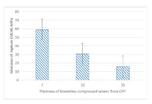
Fig. 1: Relationship thickness of binderless compressed veneer panel with  $\ensuremath{\mathsf{MOR}}$
