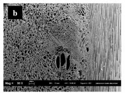
Fig. 3 (a) & (b): Scanning electron microscopy micrographs of binderless compressed veneer panel of oil palm trunk with thickness 7 mm
