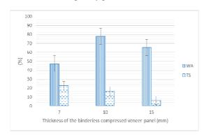
Fig. 2: Relationship thickness of binderless compressed veneer panel with water absorption and water absorption
