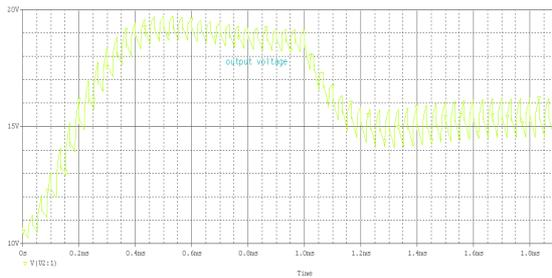
Fig.8 output voltage using switch model
