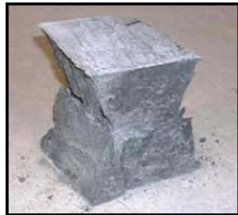
Fig. 6 Failure mode of specimen normal concrete
