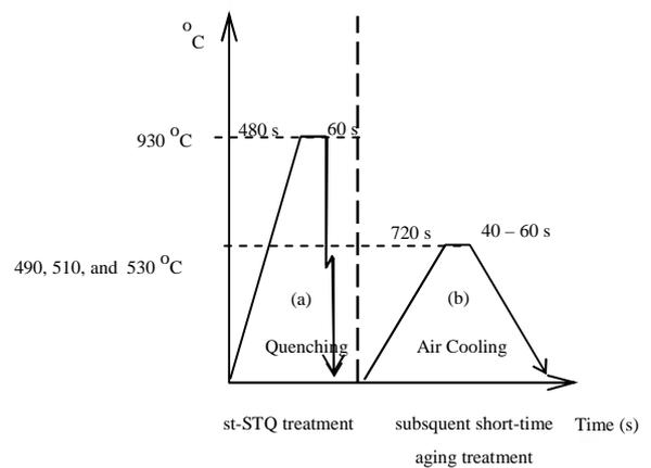
Fig. 2. Conditions of (a) short-time solution treatment and (b) subsequent short-time aging
