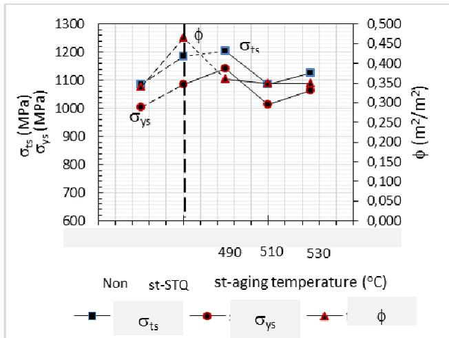
Fig. 7 Change in mechanical properties of Ti-6Al-4V with short-time solution treatment and subsequent short-time aging for 60 s.
