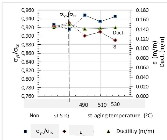
Fig. 8 Change in yield ratio, elongation and ductility of Ti-6Al-4V alloy with short-time solution treatment and subsequent short-time aging for 60 s.
