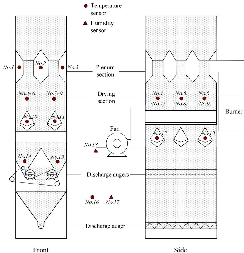
Fig. 5 The positions of temperature and humidity sensors.
