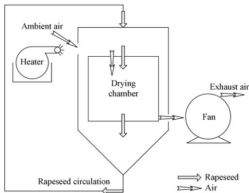
Fig. 1. Block diagram of rapeseed concurrent flow dryer.
