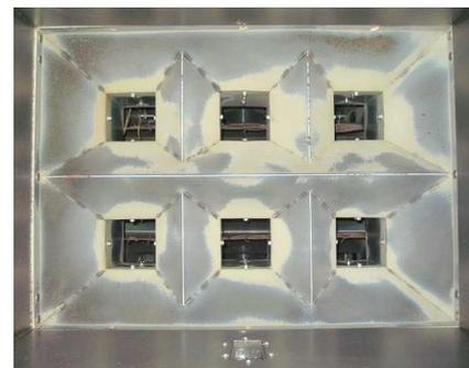
Fig. 3. View of inlet section (Y-chute type)
