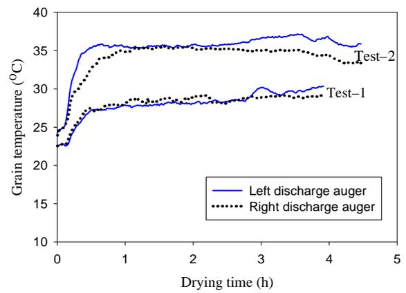
Fig. 7 Rapeseed temperature during drying at discharge augers.
