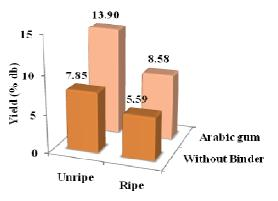
Fig 1. Effect of maturation degree and binder treatment on yield of spraydried areca nut extracted powder.
