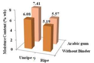
Fig 2. Effect of maturation degree and binder treatment on moisture content of spray-dried areca nut extracted powders [22].
