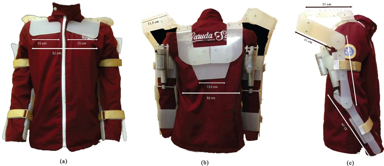
Fig. 1 The Exoskeleton of post-stroke rehabilitation device (a) front (b) back (c) left/right
