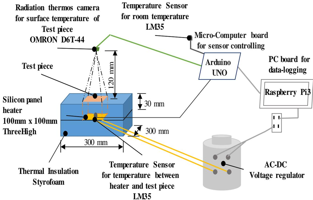
Fig .2 Components of thermal conductivity measurement system using Arduino and Raspberry Pi3
