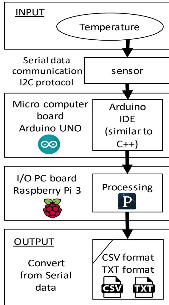
Fig.8 Data flow from sensor
