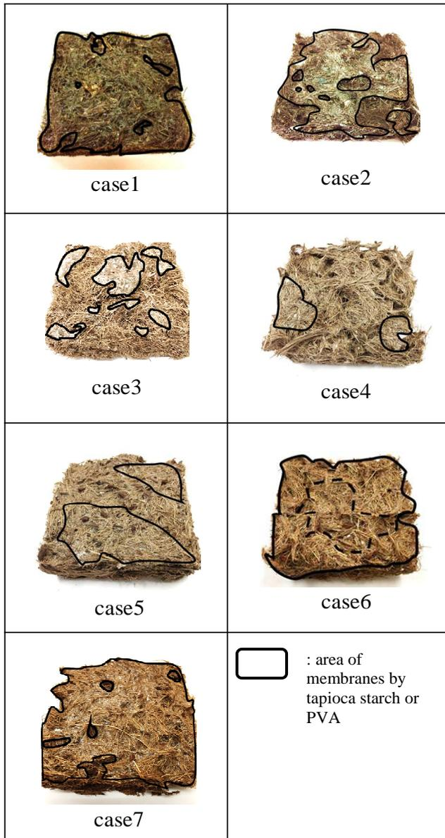
Fig.11 Membrane on test pieces
