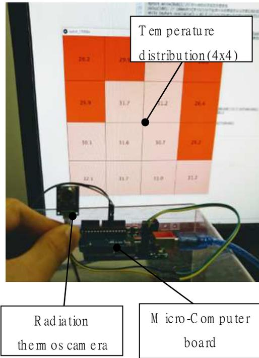
Fig.7 Temperature distribution using radiation thermos camera (OMRON D6T-44)
