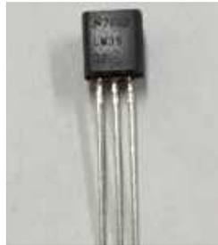
Fig.5 Temperature sensor LM35
