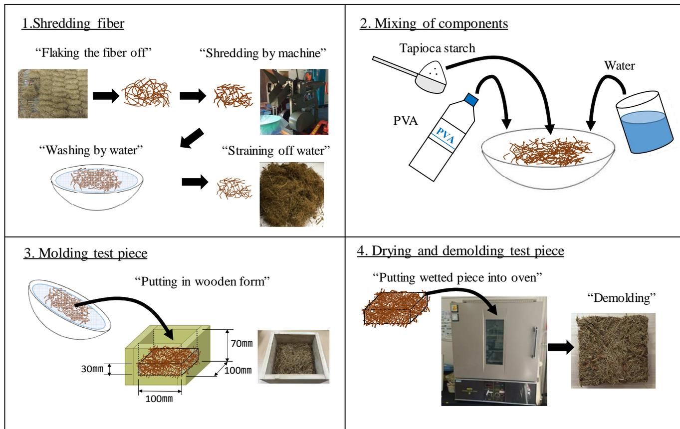
Fig 1. Process of making test pieces
