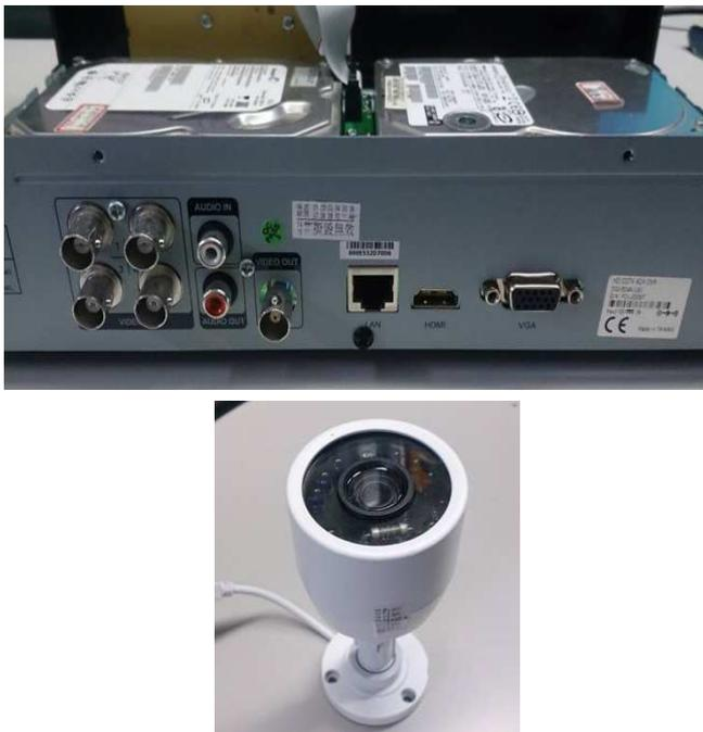
Fig. 3 IR CCTV camera and DVR system
