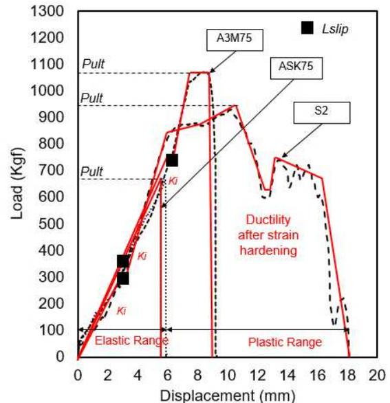
Fig. 9 Stress-strain diagram; S2-A3M75-ASK75
