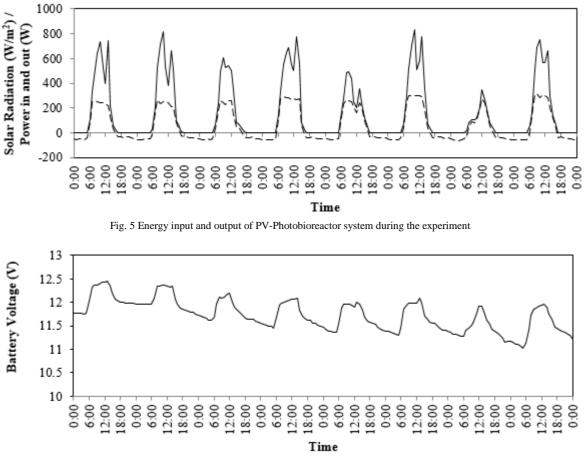
Fig. 6 Battery Voltage monitoring during the experiment
