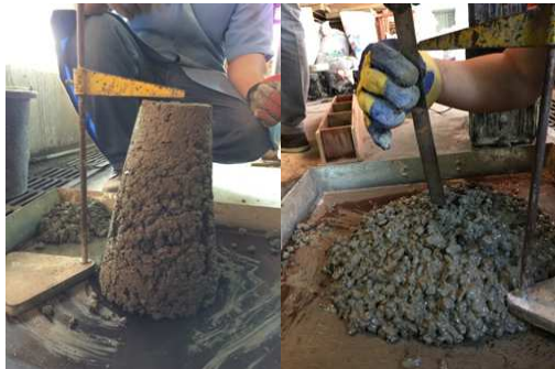
Fig. 2 Slump test without SP (left) with SP (right)
