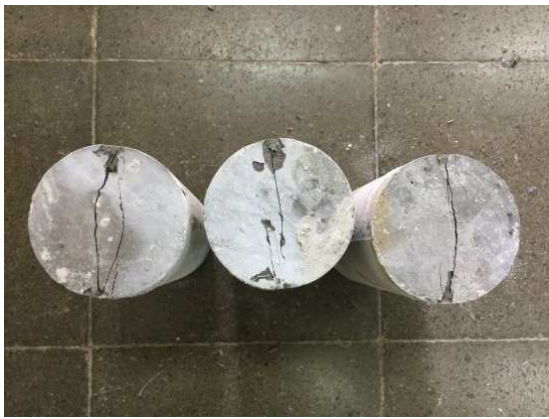
Fig. 5 Post-Test Tensile Split Specimen
