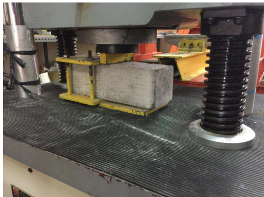
Fig. 6 Shear Test Setup on UTM
