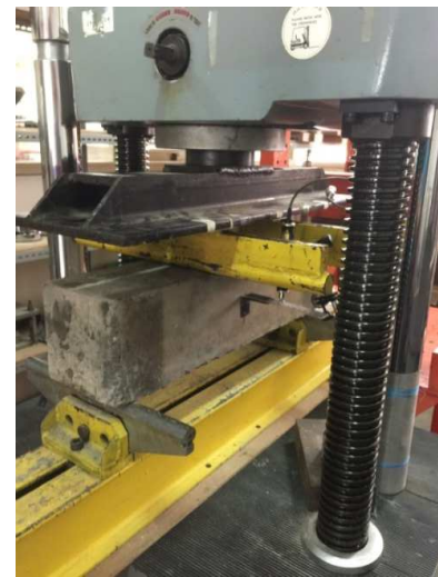
Fig. 8 Flexural Test Setup on UTM
