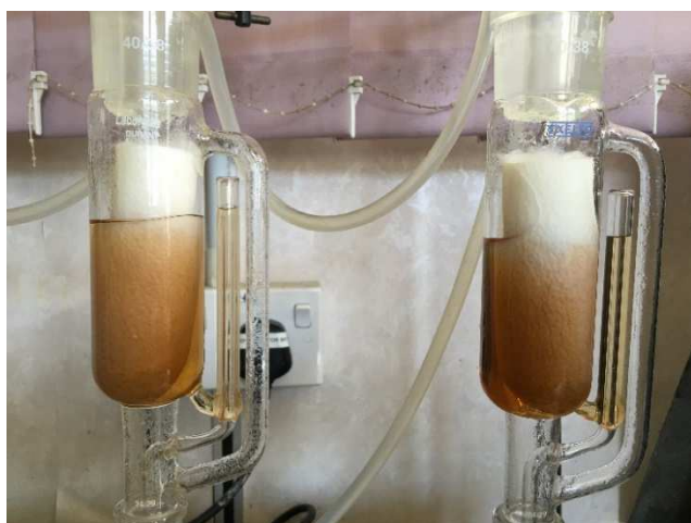
Fig. 3 Extraction chamber with the thimble
