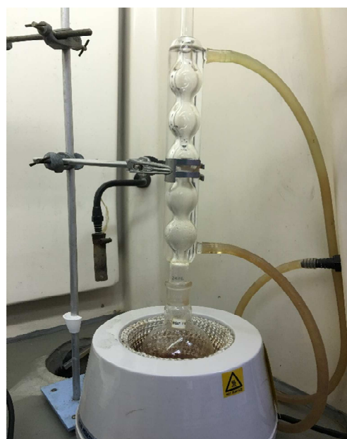
Fig. 5 Reflux setup for condensed tannin characterization
