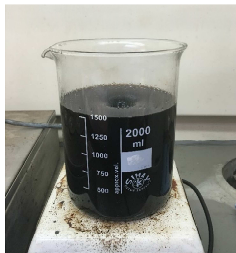
Fig. 4 Extraction by boiling
