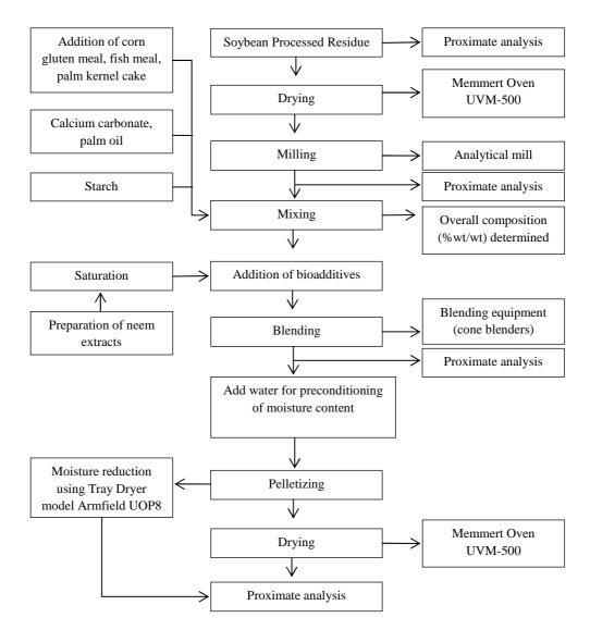
Fig. 1 Process flowchart of producing soybean pellet feedstuffs
