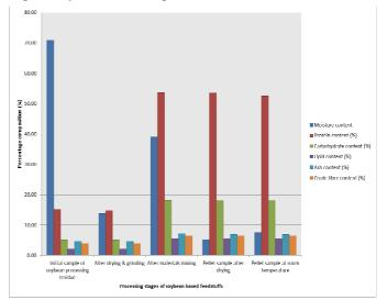
Fig. 2 Analysis of composition at different processing stages of soybean based feedstuffs
