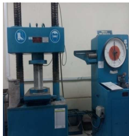
Fig. 6 Compressive test on cylinder
