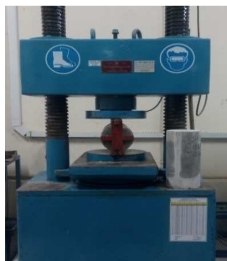
Fig. 7 Splitting tensile test on cylinder
