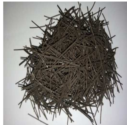
Fig. 4 The 1 inch length of steel fiber extracted from waste tyre
