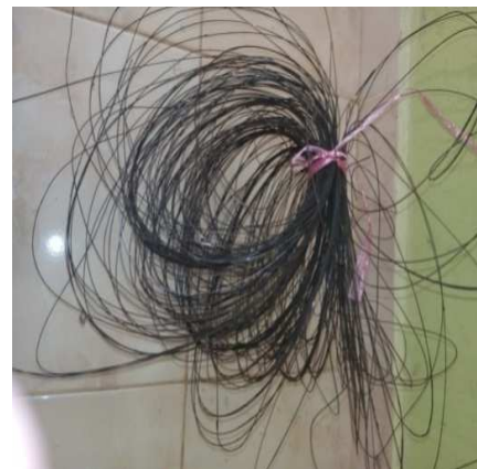
Fig. 3 Steel fiber extracted from waste tyre
