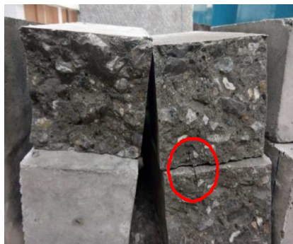
Fig. 12 Crack growth on concrete
