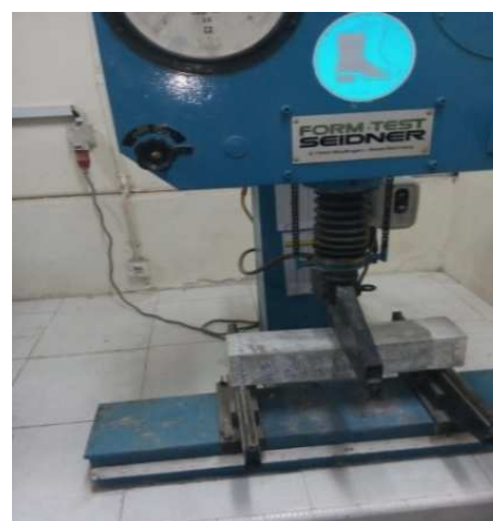
Fig. 8 Flexural test on beam
