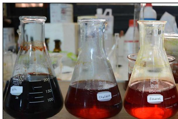
Fig. 4 The colour of the dye solution after mangosteen pericarps extraction using different solvent. Left to right: ethanol containing 1% HCl, ethanol containing 1% acetic acid, and dry ethanol
