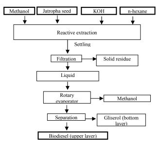
Figure 1. Experimental procedure
