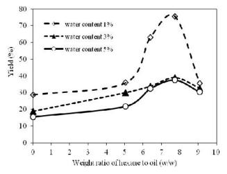
Figure 2. Effect of process parameter on yield of biodiesel
