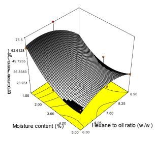
Fig.3. Combined effect of moisture content of jatropha seed and hexane to oil weight ratio on yield of biodiesel
