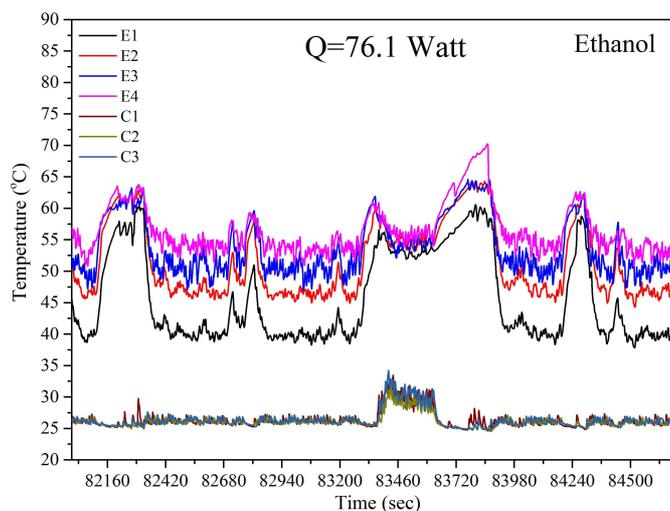
Fig. 3 Temperature fluctuation at ethanol OHP at 76.1 Watt
