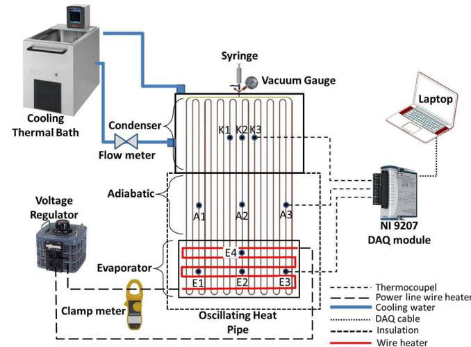
Fig. 1 Schematic of experimental setup and thermocouple locations
