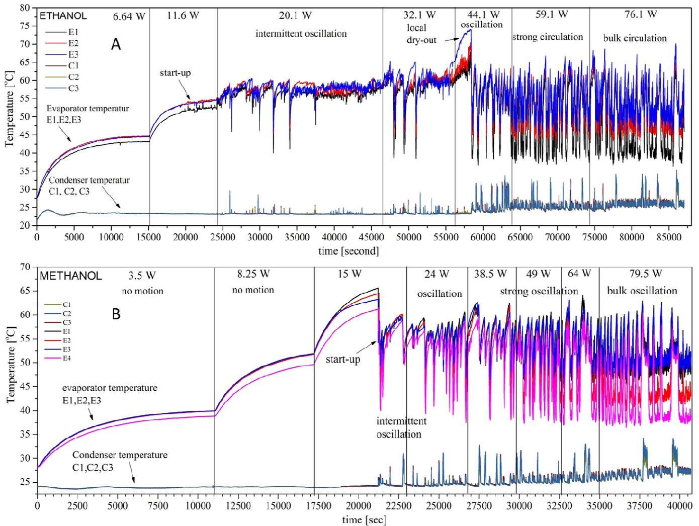
Fig. 2 Temporal evolution of evaporator and condenser wall temperature for ethanol (A) and methanol (B)
