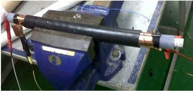
Fig. 5 Sample of 1 m XLPE cable section, prepared for PDC measurement
