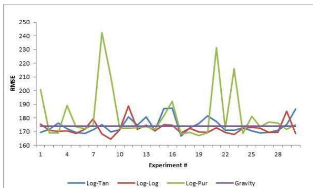
Fig. 3 NN Model testing performance/RMSE (Sigmoid nonlinear data transformation) compared with DCGM
