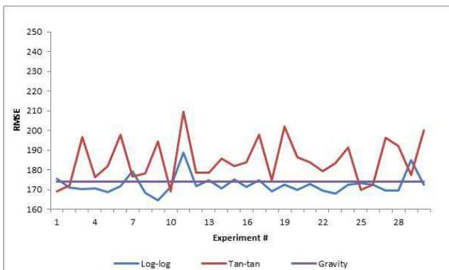
Fig. 5 NN Model testing performance/RMSE (Sigmoid and Tansig nonlinear data transformation) compared with DCGM
