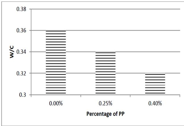
Fig. 6 Optimum w/c ratio vs. percentage of PP
