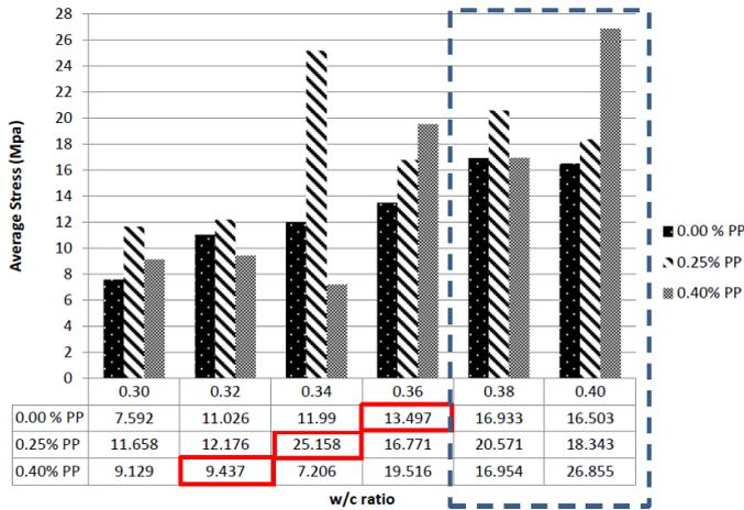
Fig. 3 Average compressive stresses vs. w/c ratio
