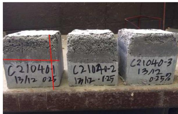
Fig. 2 Layers formed due to segregation
